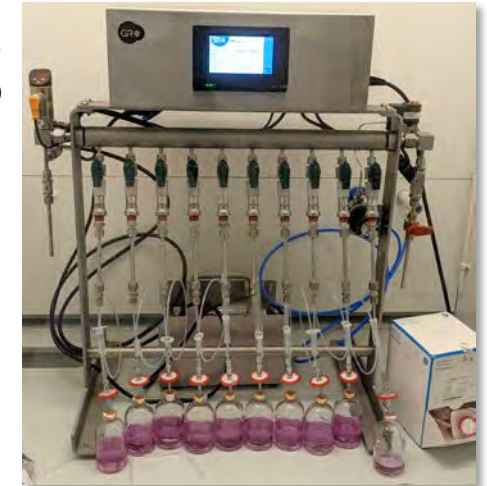
Fig. 2: To apply a 80:20 mixture of H_2:CO_2 into serum flasks, a gas-exchanger is needed (right). This instrument allows for precise application of different gases into serum flasks and enables the assessment of carbon utilisation via product formation/gas consumption. (Below), a preliminary experiment showing favourable gas consumption with Excello 90 as the sugar substrate supplement. Particularly good growth is observed in the presence of Excello 90 and H_2:CO_2 gas.
